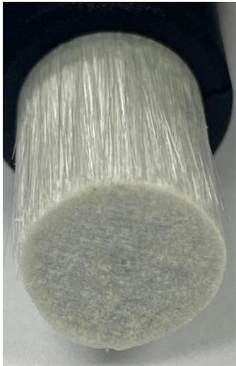
After 3-4 years of equivalent UV exposure, uncoated rods showed fully exposed fibers.
